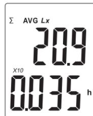
In average integral interface, the upper half of the screen shows the average illuminance in unit of  $Lx$  or  $Fc$ , the lower part shows the time for integration, in unit of hour (h).
