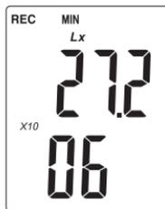
"MIN" at the top of screen means that the maximum storage groups in current manual storage area is up to 60; The upper part shows the current saved value of illumination, the lower part shows the current storage number of data.
