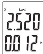
In integral interface, the upper half of the screen shows the integral of illumination in unit of  $Lx \cdot h$  or  $Fc \cdot h$ , the lower part shows the time span for integral, in unit of hour (h).
